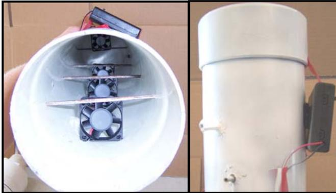
Figure A1.4: Left panel – fans inside the community chamber ensured air circulation. Right panel – a view of one of the ports that connect to the LI-COR. (Photos: Hill)
