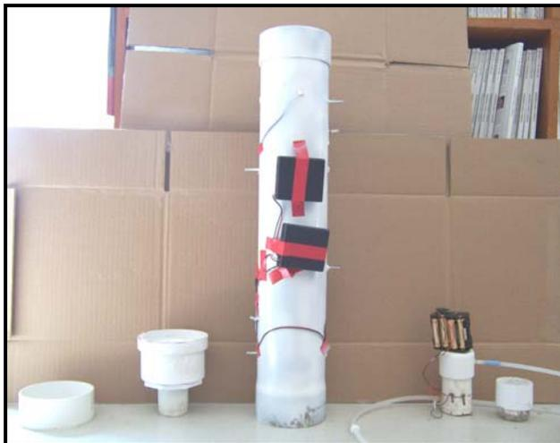
Figure A1.1: The methods used to obtain CO<sub>2</sub> flux data. From left to right, an original soil collar, a modified soil collar, the community chamber, and the mini-chamber (with its soil adapter). (Photo: Hill)
