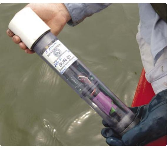
IN 2006, Project *Limulus* also started using an underwater tracking device called a submersible ultrasonic receiver, which is anchored underwater, and can pick up the sonar tag frequencies within 400 meters.
