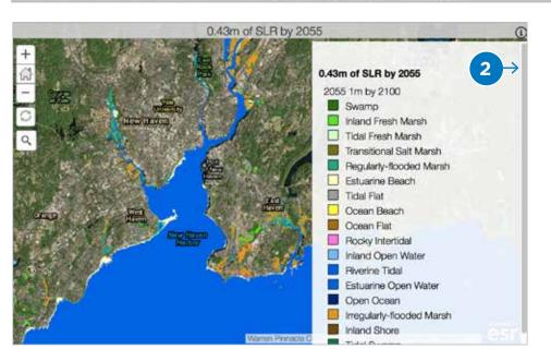
2 A map view with the SLAMM land-cover classification legend frame displayed. Notice the scroll bar on the right side of the frame that can be moved up or down to see additional classes and color schemes. The legend frame not only identifies the land cover, but also reiterates the SLR conditions (0.74 m by 2055) and provides the model scenario used (2055 Rapid Ice Melt Maximum).
