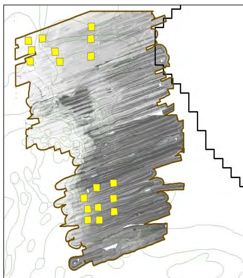
Figure 5.1-4: Side scan mosaic produced by Twichell et al. (1998) located on the eastern flank of the pilot study area; yellow boxes show areas sampled by Zajac (1998) for two years to look at seasonal and yearly changes in benthic community structure in relation to the various seafloor habitat elements found within the mosaic area.
