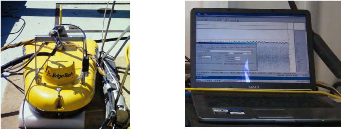
Figure 4.5: Lamont EdgeTech Chirp 424 subbottom profiler system (left) and EdgeTech Discovery software (right).
