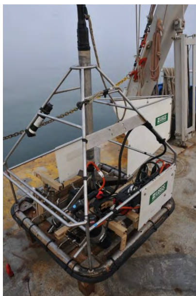
Figure 5.2-5: SEABOSS used to collect sediment samples, photos, and videos of the seafloor. (Photo: Dann Blackwood; Blackwood and Parolski, 2001)
