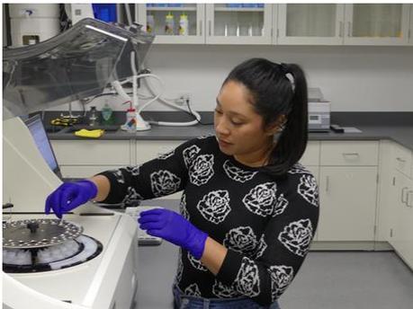
Elena Colon, laboratory manager at the Unified Water Study's laboratory in Larchmont, New York, places sample cups into the facility's new discrete analyzer. The new equipment enables the UWS to do in-house analysis of water quality samples for nitrogen, phosphorous, continuous dissolved oxygen, and additional measures. (LISS photo/Robert Burg)
