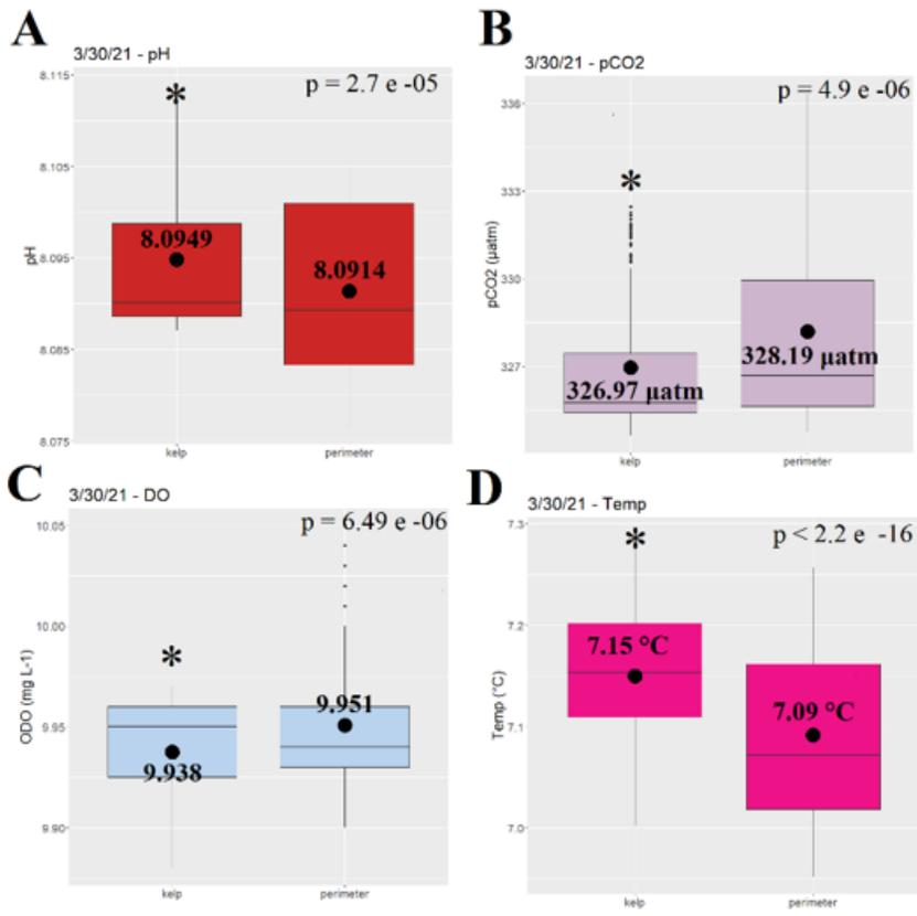
Figure 3e.4. Combined flow-through data from the 3/30/21 cruise, showing pH (A), pCO<sub>2</sub> (B), dissolved oxygen (C), and temperature (D). Large dots on boxplots indicate mean value, with mean value shown in text bolded near dots. Asterisk indicates statistically significant difference between the within-kelp field and perimeter for that parameter.
