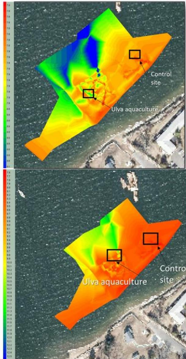
Fig 3e8. Surface pH (above) and DO (below) levels mapped around a 25-bag Ulva array deployed in Northport Harbor as depicted in Figure 2C2 by a Hycat autonomous surface vehicle equipped with a YSI EXO3 sonde.
