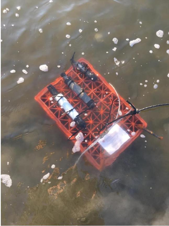
Sensors monitoring conductivity, pH, and DO continuously in Northport Harbor.
