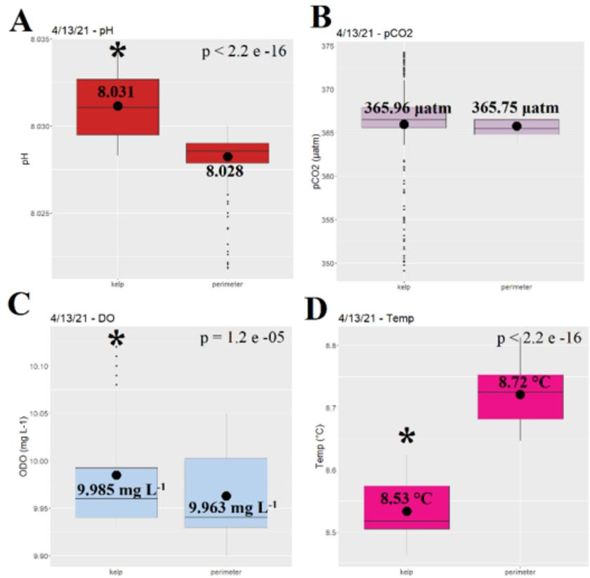
Figure 3e.5. Combined flow-through data from the 4/13/21 cruise, showing pH (A), pCO<sub>2</sub> (B), dissolved oxygen (C), and temperature (D). Large dots on boxplots indicate mean value, with mean value shown in text bolded near dots. Asterisk indicates statistically significant difference between the within-kelp field and perimeter for that parameter.
