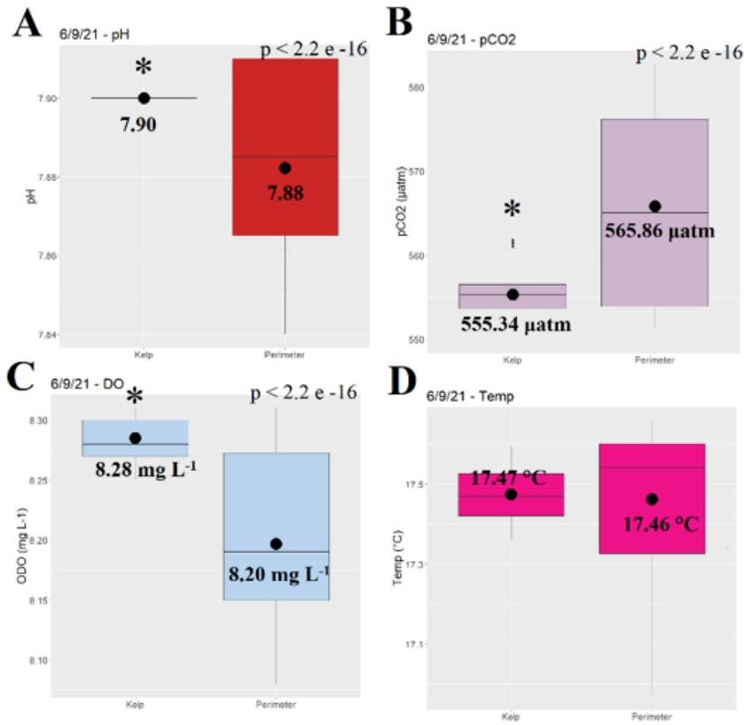
Figure 3e.7. Combined flow-through data from the 6/9/21 cruise, showing pH (A), pCO<sub>2</sub> (B), dissolved oxygen (C), and temperature (D). SeaFET sensor was malfunctioning for this cruise, so EXO pH data is displayed instead. Large dots on boxplots indicate mean value, with mean value shown in text bolded near dots. Asterisk indicates statistically significant difference between the within-kelp field and perimeter for that parameter.
