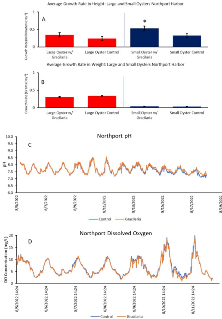
Figure 3d.9. Comparisons of (A) height-based oyster growth rates (B) weight-based oyster growth rates, (C) seawater pH, and (D) seawater dissolved oxygen in areas where oysters are co-cultivated with *Gracilaria* and control areas where oysters are grown without *Gracilaria*, in the Northport Harbor experiment in 2022. Initial timepoint to final timepoint was 13 days. Error bars indicate standard error. Asterisks indicate significant differences from control group.
